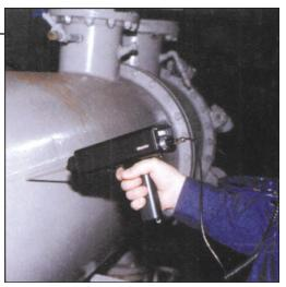
**FIGURE 3.** Fluid leaking from tubes of a heat exchanger can be heard from the outside without interrupting operation
