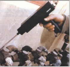
FIGURE 2. A simple contact of the probe will test a steam trap
